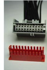
Un-damaged TPA after removal
