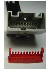
Un-damaged TPA after removal
